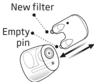
Insert the empty pin into the wax filter in the earpiece and pull it out.
