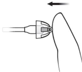
Push firmly to ensure that the earpiece is securely fastened.
