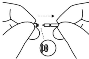
3. Pull the tool straight out – your new wax filter will remain in place. Re-attach your dome or a replacement dome.
