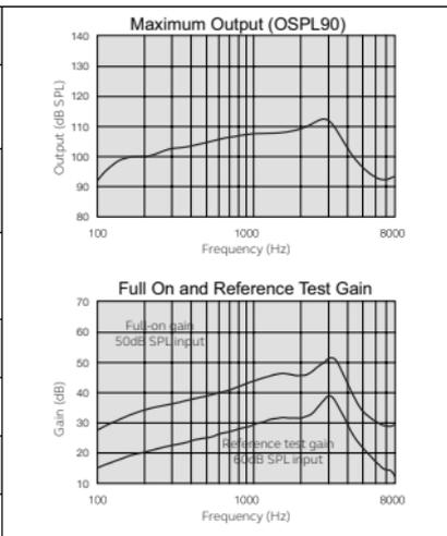
Data in accordance with ANSI S3.22-2014, IEC 60118-0:2015. Measured in a 2cc coupler.
