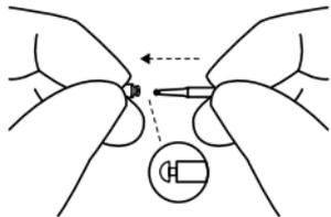
3. Insert the removal tip into the used wax filter and then pull the tool straight out. It is important to pull it straight and not on an angle.
