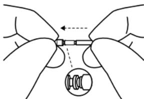
2. Gently press the replacement straight into the sound outlet until the outer ring is touching the sound outlet.
