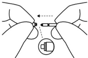
1. Insert the other end of the tool into the sound outlet (the end with the replacement filter).
