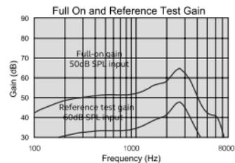
Data in accordance with ANSI S3.22-2014, IEC 60118-0:2015. Measured in a 2cc coupler.
