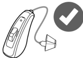
3. Check that the tulip dome is securely mounted by verifying that the collar completely covers the ribbed end of the receiver.
