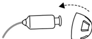
2. Push the new dome over the ribbed end of the receiver.
