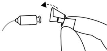
1. Remove the used dome by pulling it off the receiver and discard. This may require a bit of force.
