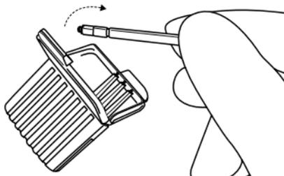
2. Open the wax filter case and take out one of the tools. Each tool has a small hook (removal tip) in one end and a new wax filter in the other.
