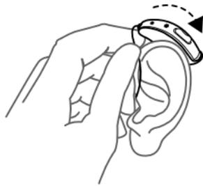
1. Hold the earmould between your thumb and index finger and position the sound outlet into your ear canal.
