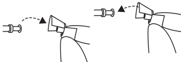
1. Remove the used dome by pulling it off the ribbed end and then discard it. This may require a bit of force.
