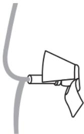
3. Check that the tulip dome is securely mounted by verifying that the collar completely covers the ribbed end of the receiver.
