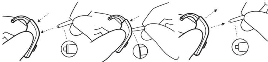
1. Insert the other end of the tool (the end with the replacement filter) into the microphone opening.
