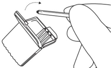
2. Insert the removal tip into the used microphone filter and then pull the tool straight out. It is important to pull it straight and not on an angle.
