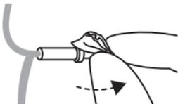
3. Check that the dome is securely mounted by carefully lifting the lower part of the dome and verifying that the collar completely covers the ribbed end.
