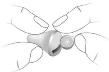
Inserting the battery:
