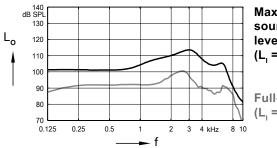
Max. Output sound pressure level  $(L_1 = 90 dB)$
